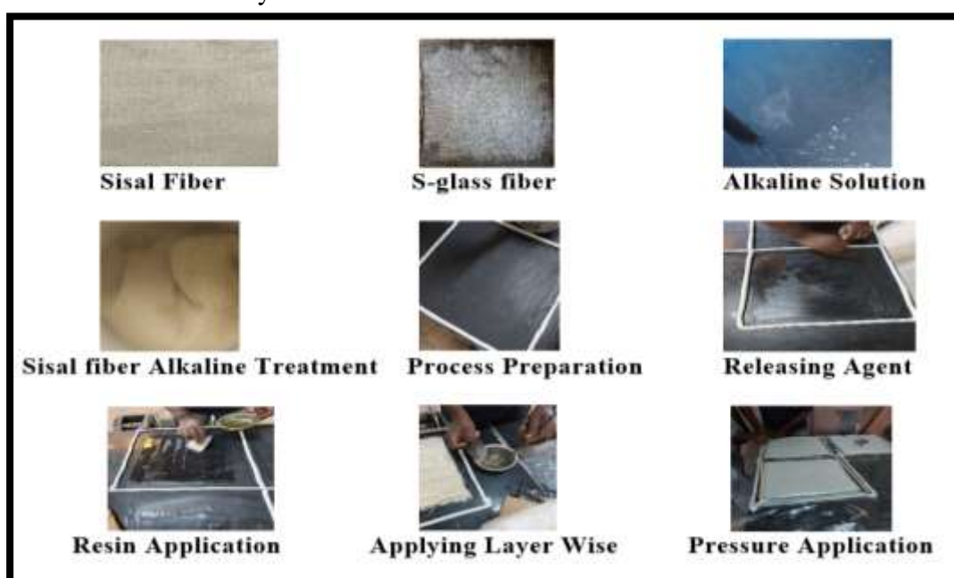
Figure 2. Pictorial of the fabrication process
