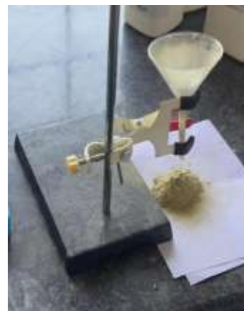
FIG 2.2 Angle of repose
