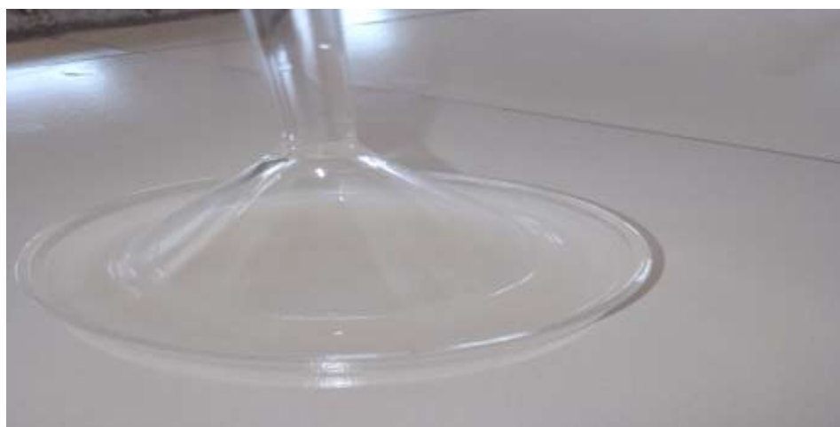
Fig 1.3- petri dish is covered with inverted funnel
