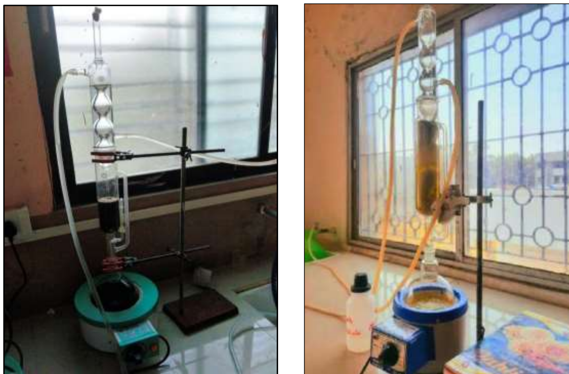
Figure 1: Soxhlet extraction of Aegle marmelos fruit & Trigonella Trigonella foenum seeds
