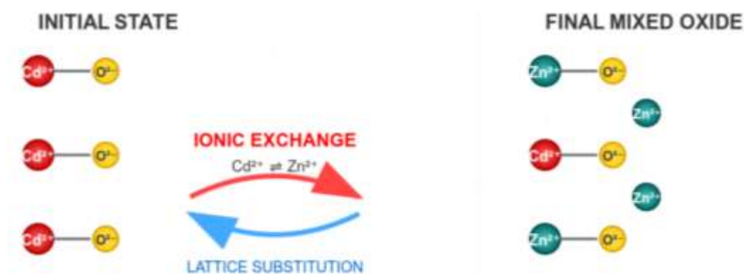
Figure 9. Ionic exchange mechanism in CdO-ZnO nanocatalyst showing lattice substitution of \text{Cd}^{2+} ions by \text{Zn}^{2+} ions, resulting in mixed oxide formation with enhanced catalytic properties.
