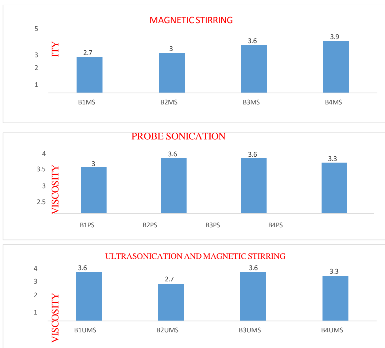
Fig:14 A graph illustrating the viscosity range of various mouthwash formulations loaded with different bases, obtained through the Magnetic stirring, probe sonication, Ultrasonication, and magnetic stirring method, is presented
