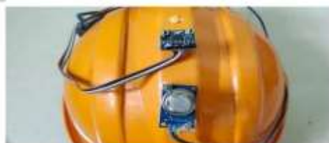
Fig 3. Lab tests showed accurate detection of temperature increases, smoke, fire, and gas concentrations beyond thresholds.
