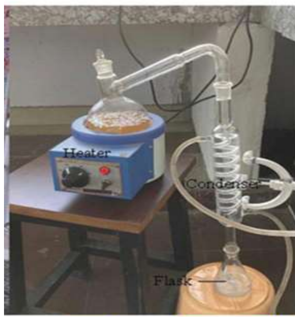
Figure 2. Setup for separation of crude water hyacinth oil with n-Hexane
