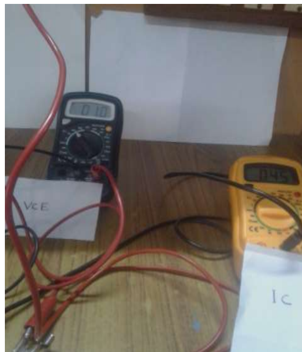
Figure 11 V_{CE} and I_C for V_{GE} = 4.90V
