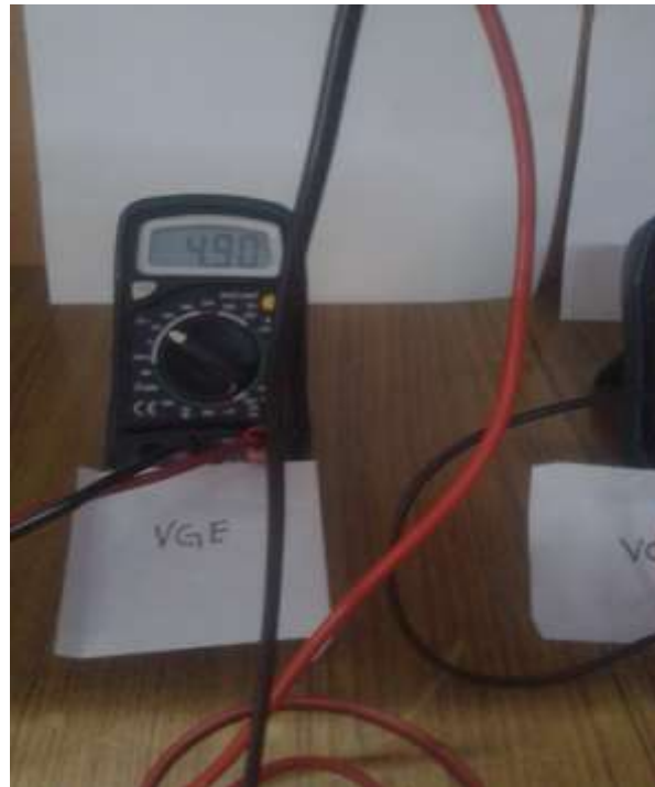
Figure 10 Gate to emitter voltage V_{GE} = 4.90V
