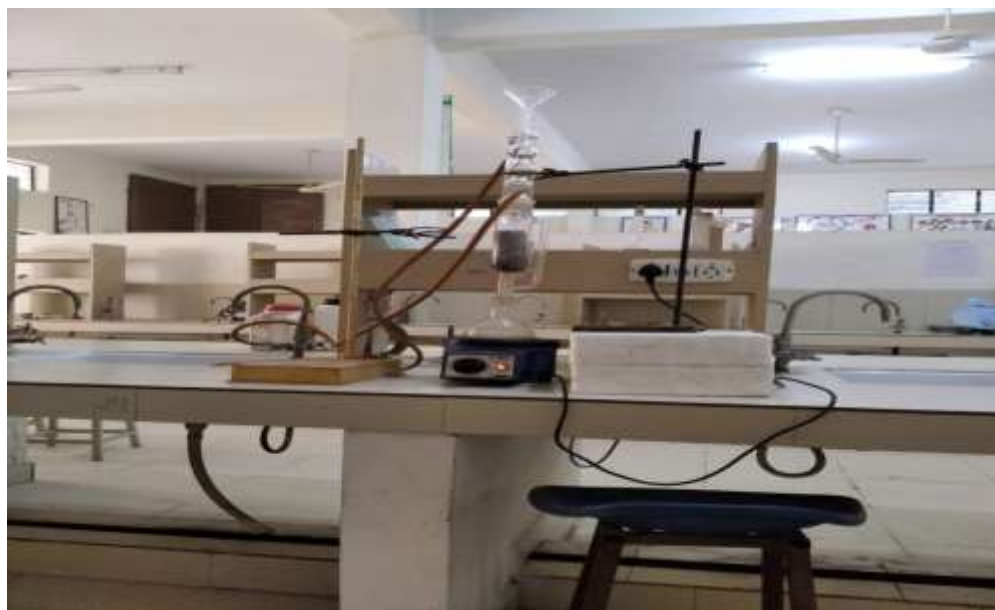
Figure: An assembly is put up to extract plant extract using the aid of a Soxhlet equipment.
