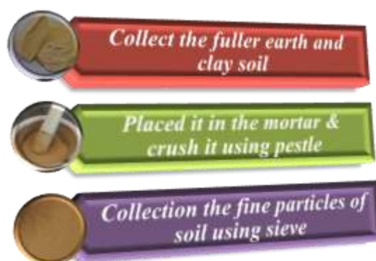
Fig.7 – Flowchart of making fine soil powder.
