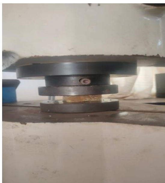
Figure 10: Compression strength testing.
