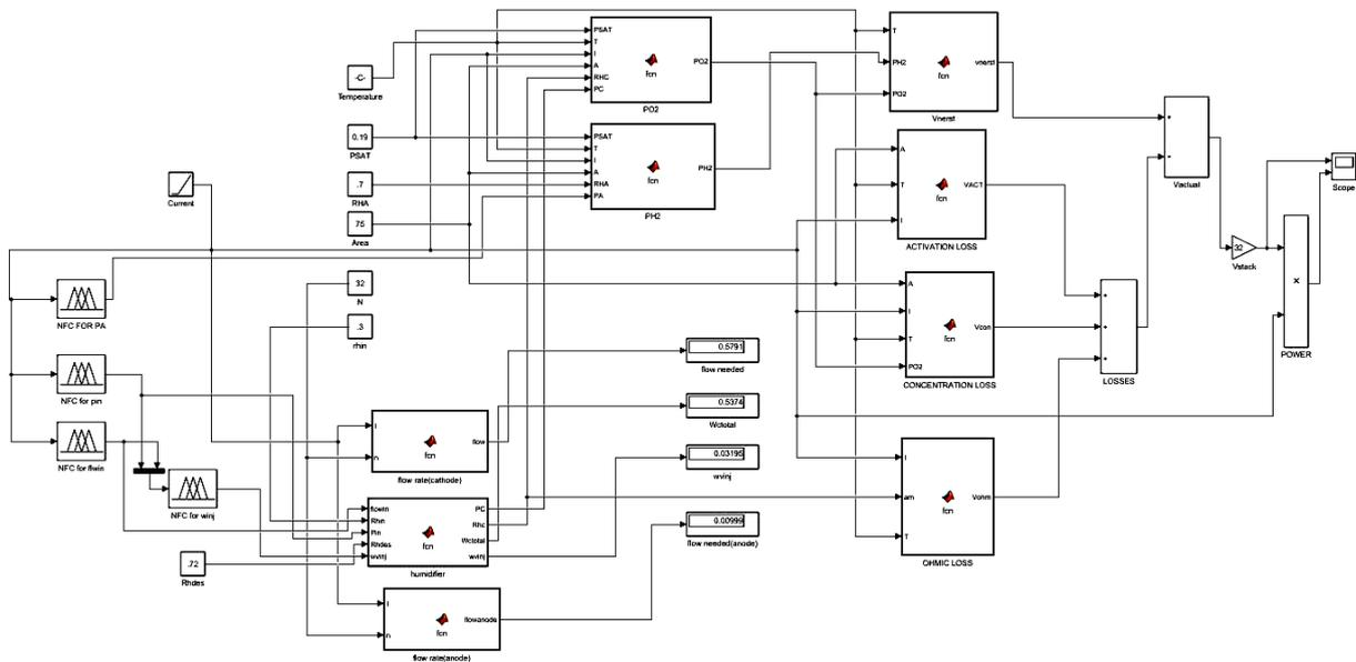
Fig 2: 500 W PEMFC Model layout in Matlab/Simulink
