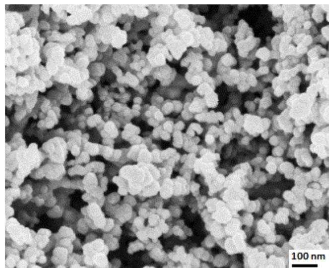
**Figure 1 SEM image of CeO<sub>2</sub> nanoparticles**
