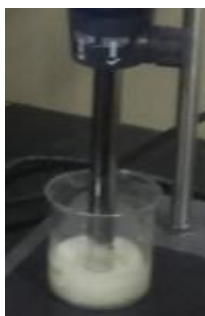
Fig.7. Formulation of o/w Nanoemulsion by High-Speed Homogenizer
