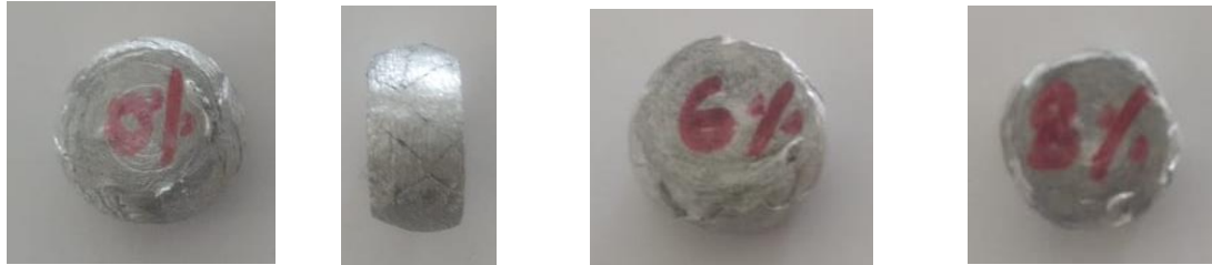
Figure 3 Specimens after compression test
