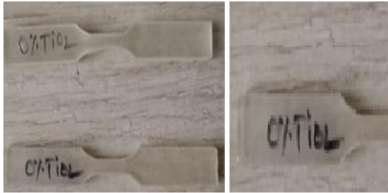
Fig.15 before & after 0% TiO 2 Tensile Specimens prepared by Nano particles
