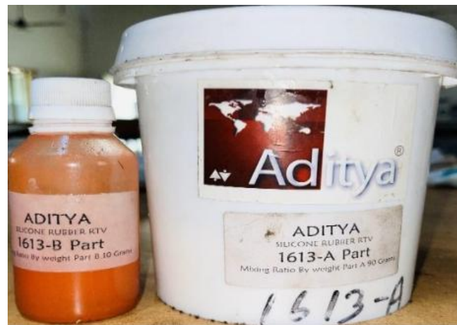
Fig.6 Silicon rubber for Rubber mold (10:1) ratio
