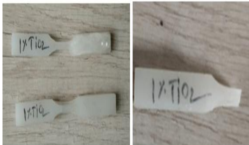
Fig.16 before & after 1% TiO 2 Tensile Specimens prepared by Nano particles
