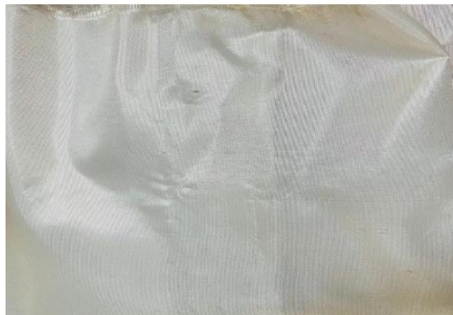
Fig.9 Glass fiber of 380 GSM
