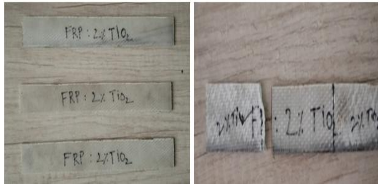
Fig.27 before & after 2% TiO_2 glass Epoxy + Resin + Hardener Specimens
