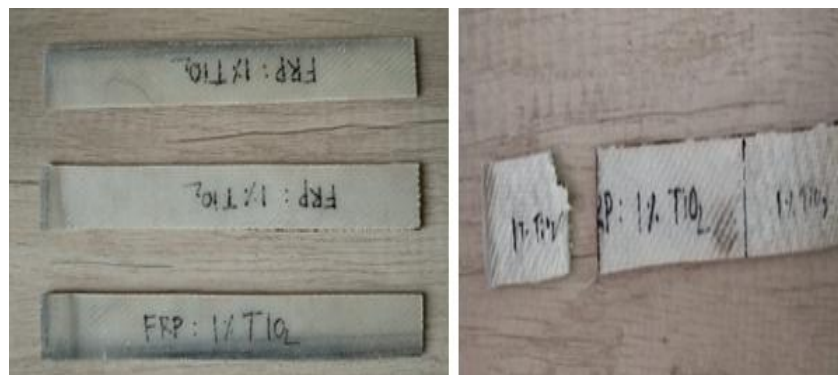
Fig.26 before & after 1% TiO 2 glass Epoxy + Resin + Hardener Specimens
