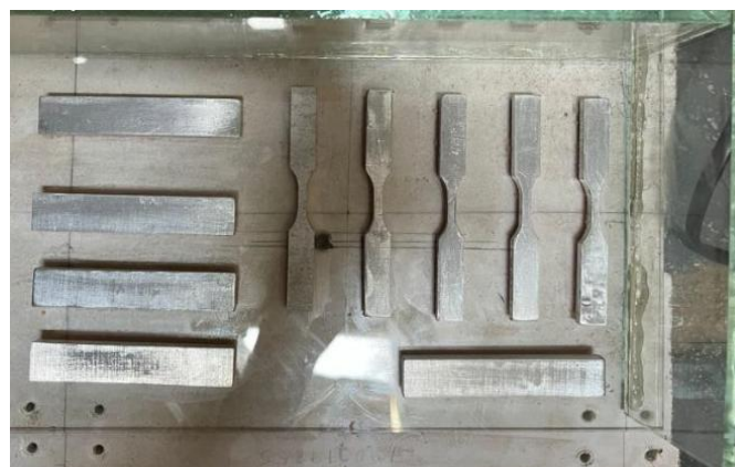
Fig.7 Aluminum patterns for making rubber mold preparation
