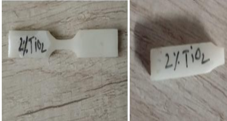
Fig.17 before & after 2% \text{TiO}_2 Tensile Specimens prepared by Nano particles
