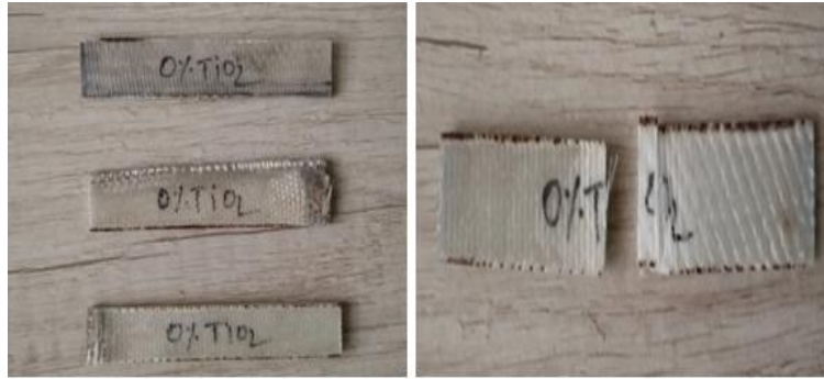
Fig.30 before and after 0%TiO 2 Impact FRP specimen
