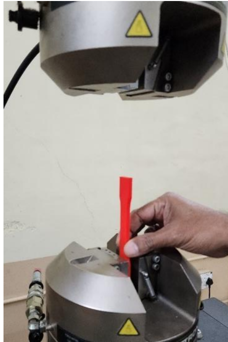
Figure 7 Arrangement of specimen for tensile test
