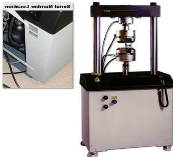
Figure 6 INSTRON 8801 Fatigue Testing Machine
