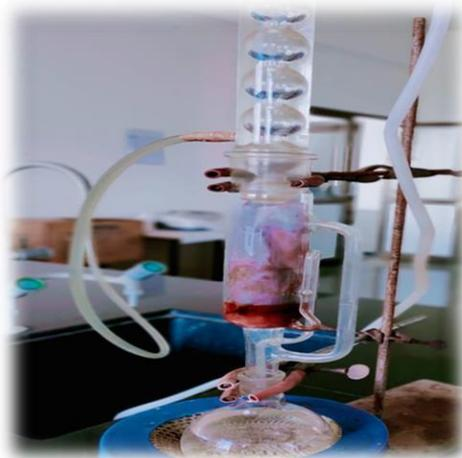
**Fig 4. Soxhlet extraction**
