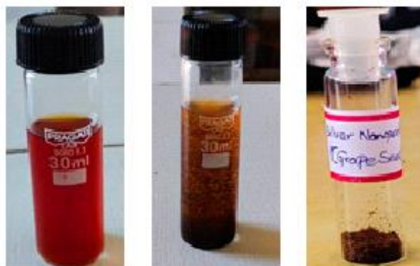
Figure. 3: Colour change of Vitis vinifera seed extract before after addition of AgNO 3 .
