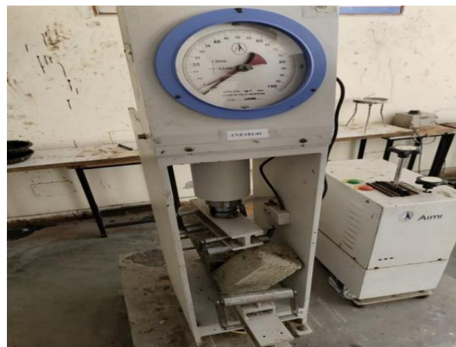
Fig. 2 Testing of Beam by FTM
