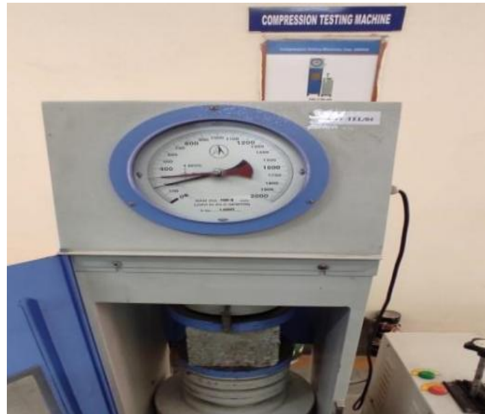
Fig 1 Testing of Cube by CTM
