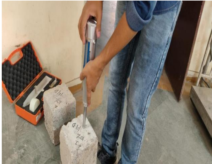
Fig 3 Rebound hammer test
