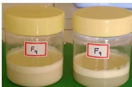
Figure 3. Phase separation of F4 and F9
