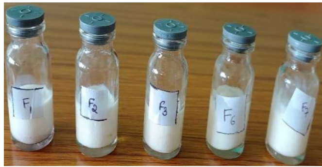
Figure 5. Formulations before H/C. No phase separation is seen
