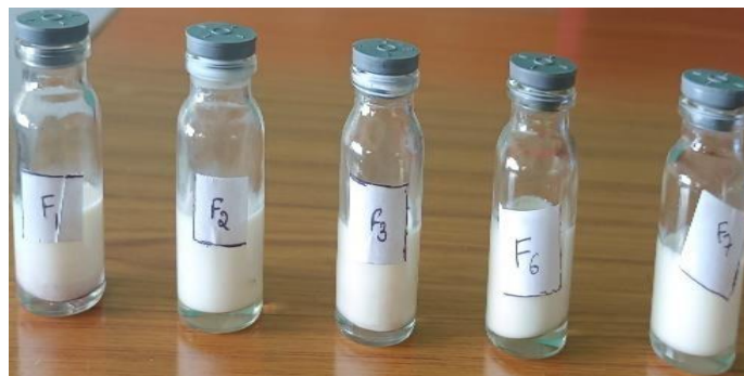
Figure 6. Formulations after H/Ccooling. No phase separation is seen cooling.
