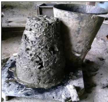
Fig. 3.1 Slump of the Concrete
