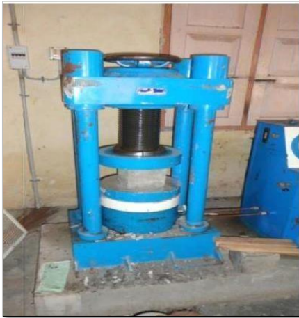
Fig. 3.2 Test setup for Compression Test on cubes
