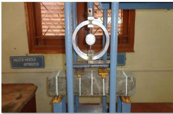
Fig. 3.4 Test setup for Flexural Strength
