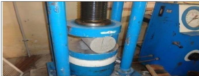
Fig. 3.3 Test setup for Split Tensile strength
