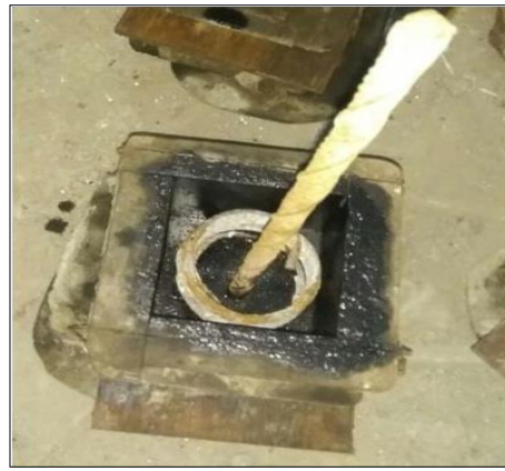
Fig. 3.6 Casting of Pullout Cube Specimen
