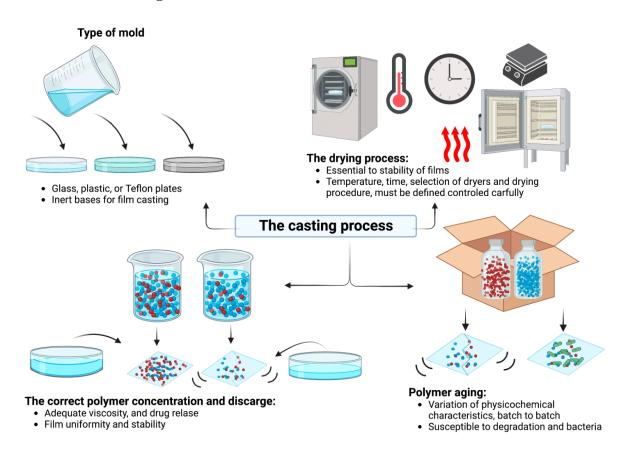
This is a very old method of film making. In this method the drug is dissolved or suspended in a solution containing polymers, plasticizers and other excipients which are dissolved in a volatile solvent such as ethanol or water.
