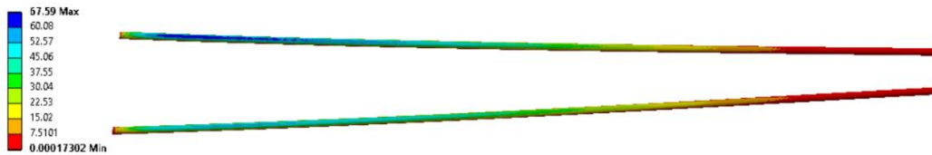
Fig. 21 Von-Mises Stress on Spar
