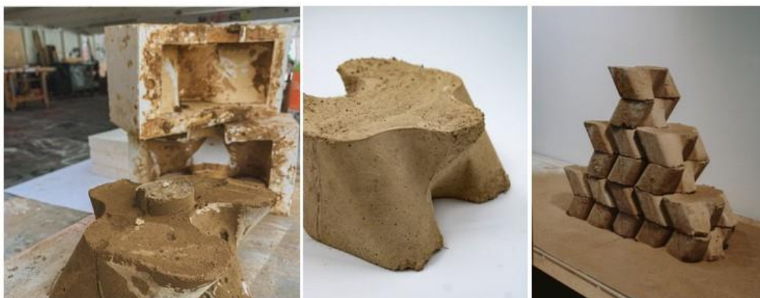
Figure 12. The phases of Terrablocks parametric adobe made with 3D printed molds
