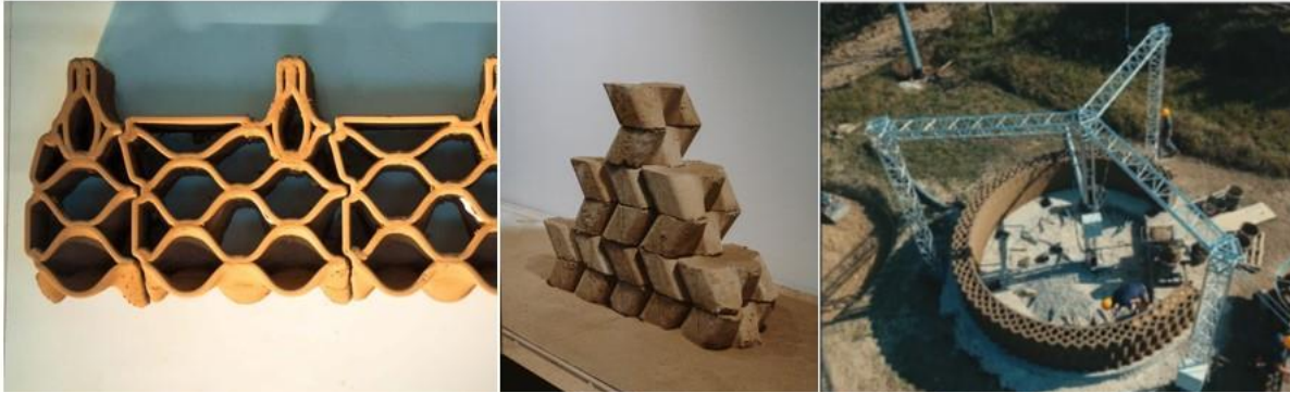
Figure 8. left: 3d printed adobe brick from Digital Adobe, middle: Terrablocks adobe bricks from 3d printed molds, right: monolithic printed wall of Gaia project by WASP
