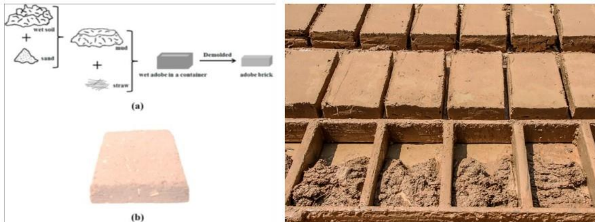
Figure 4. Steps of making traditional adobe bricks
