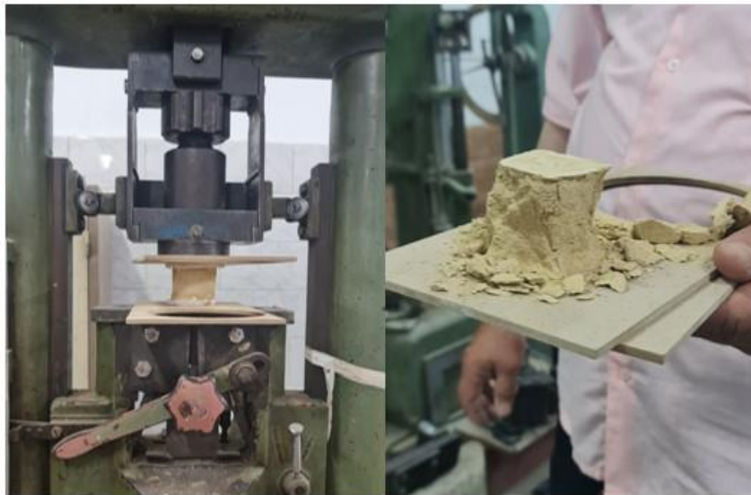
Figure 16. Universal Testing Machine conducting compression tests & failure modes in samples
