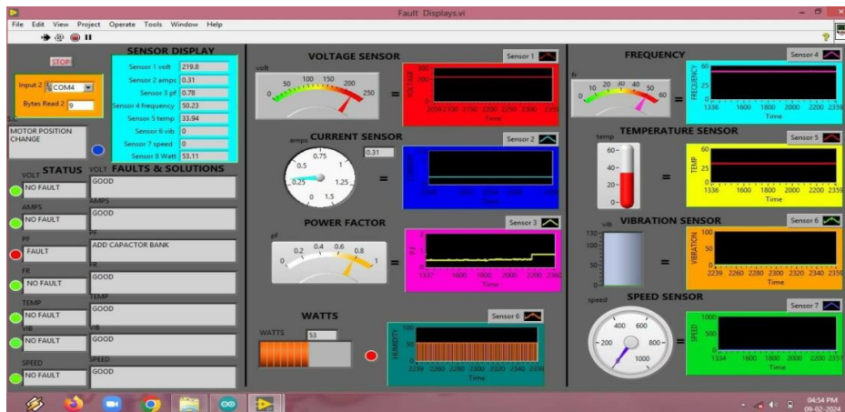
Fig.4. Dashboard of the proposed System in LabVIEW
