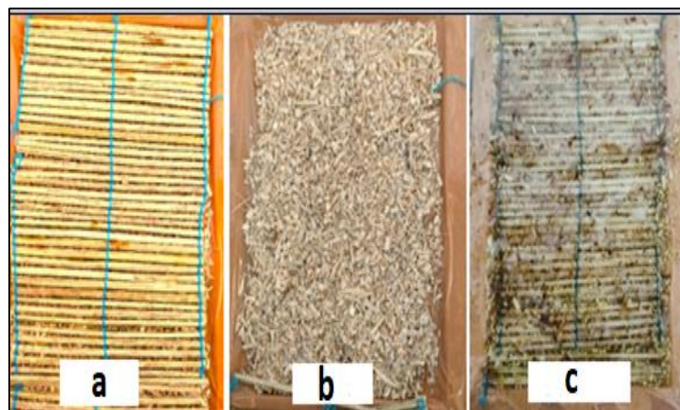
Fig.3. Fabricated Specimen 2: a) Date palm fibers, (b) Particulate form of sugarcane bagasse and groundnut shell and (c) Fabricated specimen with fibers hybridized along with epoxy and hardener
