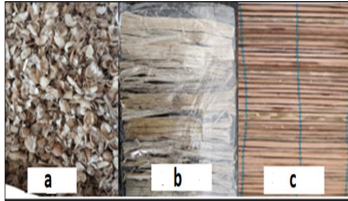
Fig.1. Constituents of Composite a) Groundnut Shell (b) Sugarcane Bagasse and (c) Date Palm fiber
