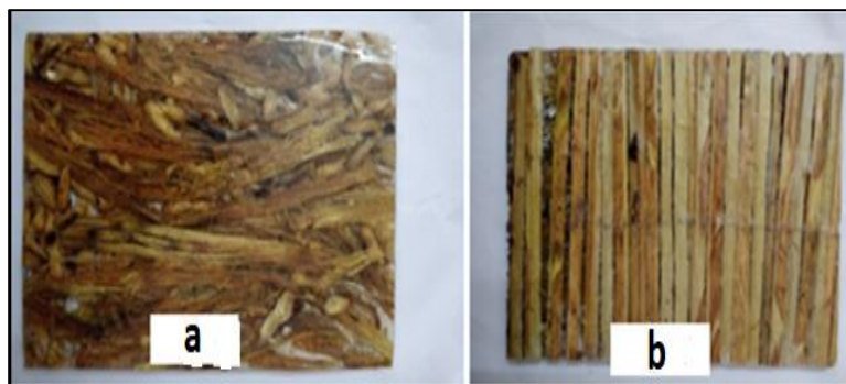
Fig.3. Fabricated Specimen 1 with fibers hybridized a) Front view (b) Back view
