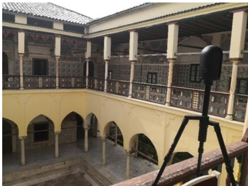
Fig.4. LEICA BLK360 Scanner in situ (Source: Authors 2022).
