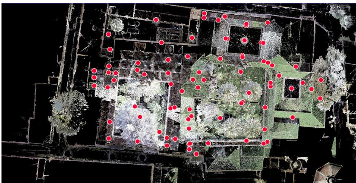
Fig.6. scan station inside the palace (Source: Authors, 2023).
