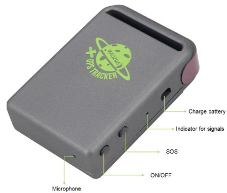
Fig. 19: TK-102B GPS pin configuration
