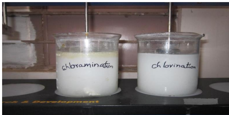
Figure 3.1: Chloramination and Chlorination during mixing.
