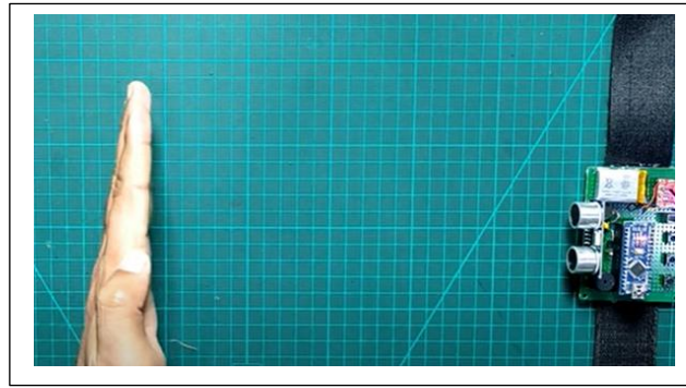
Fig.5.2. Object detection by smart gloves
