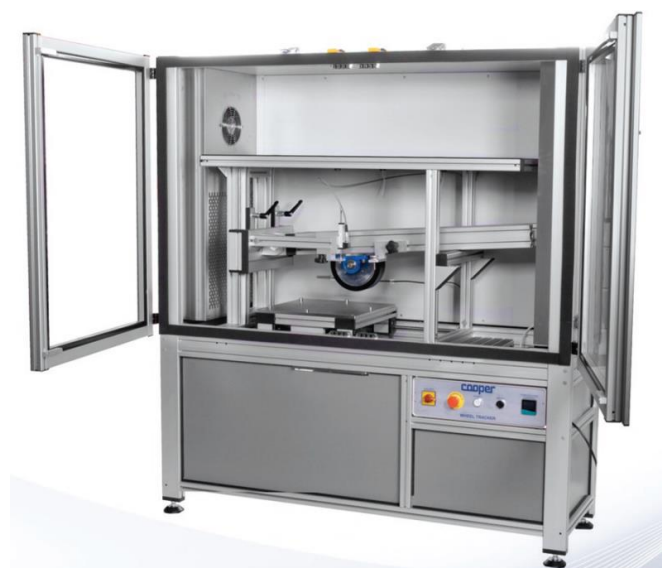
Fig. 1. Cooper wheel tracking test equipment (www.averest.com)
