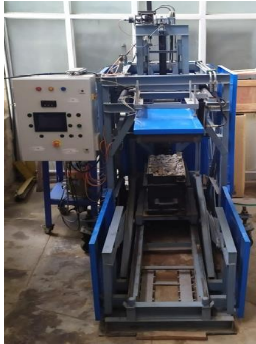
Fig. 5. Roller compactor cum rut analyser [20]
