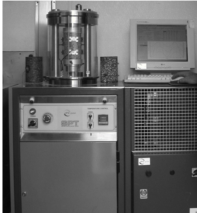
Fig. 3. Simple Performance Test (SPT) Device in FHWA Mobile Asphalt Laboratory [18]
