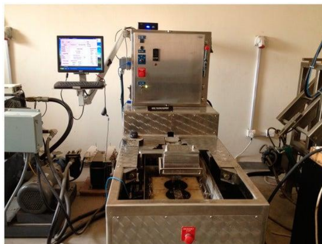
Fig. 2. Hamburg Wheel Tracking Device [16]
