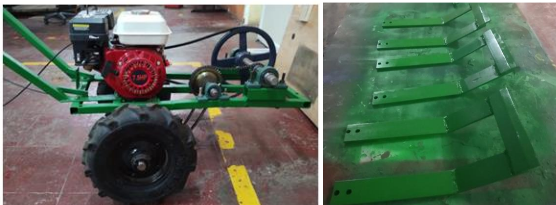
Figure 1.7 Final physical mode of groundnut weed removing machine with blades
