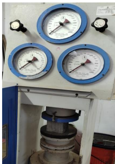
Fig. 3 Testing of specimens on CTM
