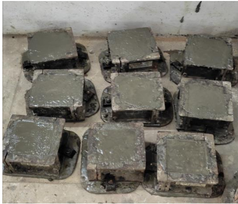
Fig. 1 Casting of specimens
