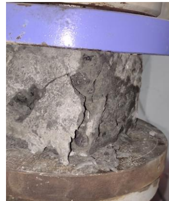
Fig. 4 Failure pattern of specimens
