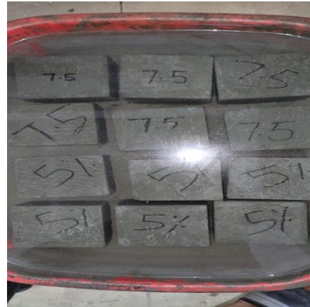
Fig. 2 Curing of specimens
