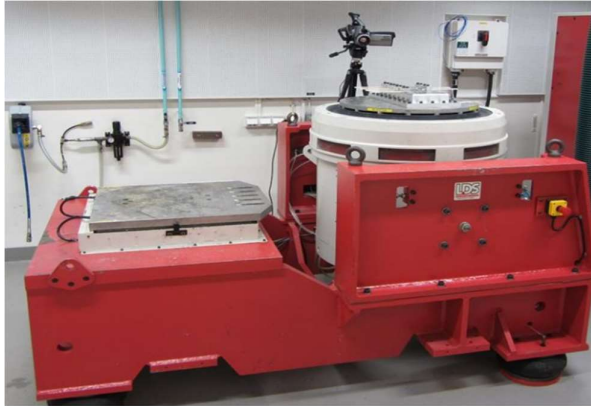
Fig.1 Electrodynamic shaker (cylindrical white piece on the right) and associated slip table (left)
