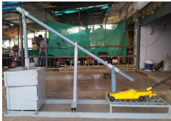
Figure 6.10 Fabricated Mini-Baler Machine
