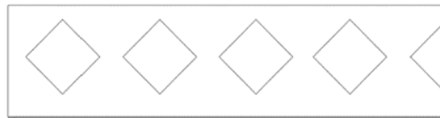
Figure 3. Castellated column with diamond opening.
