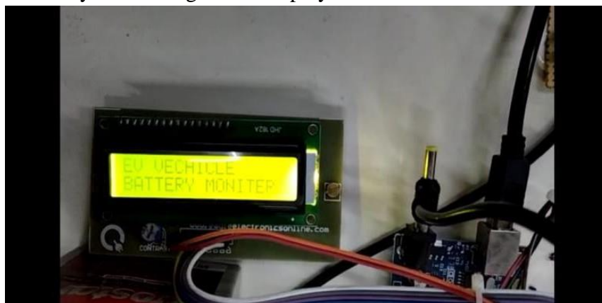
Figure (2) : EV Battery moniter
