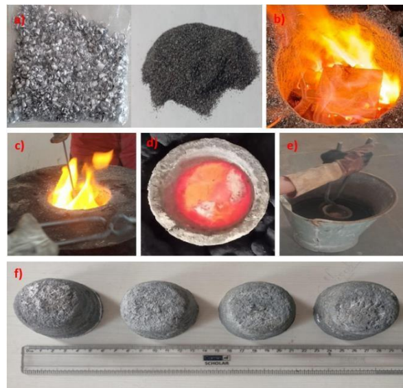
Fig 1. Steps involved in the development of the composites (a) Aluminium and MS scrap chips/powder, (b) Melting of aluminium, (c) Addition of MS powder and stirring, (d) Molten metal, (e) Ice cool water quenching for solidification and (f) Developed composites.
