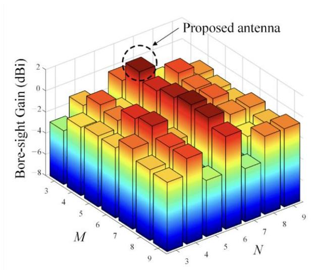
Figure 9 shows differences in bore-sight gain according on reflector count.
