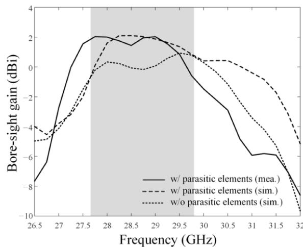
Figure 6 shows the proposed antenna's measured and simulated bore-sight gains with and without parasitic elements.
