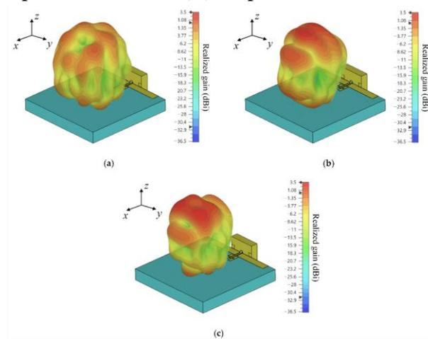
Figure 8 displays three-dimensional patterns at 26 GHz, 28 GHz, and 30 GHz.
