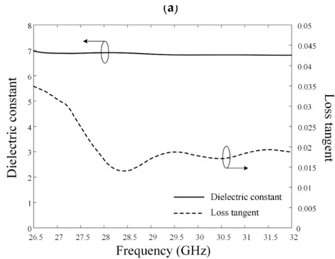
Figure 4 shows the thick car window glass substrate's measured EM properties, including (a) loss tangent and dielectric constant.
