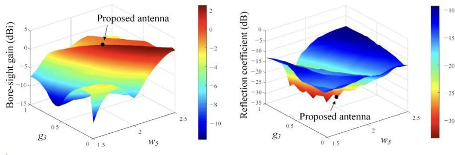
Figure 10 shows the fluctuation of the parameters  $w_5$  and  $g_3$  in relation to the bore-sight gain and reflection coefficient: (A) the gain in boresight; (B) the reflection coefficient.
