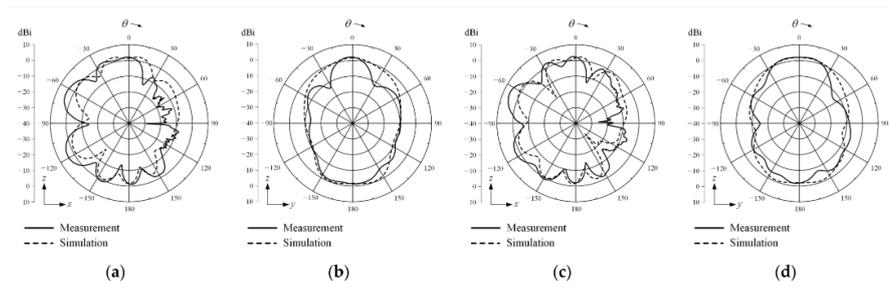
Figure 7 shows the proposed antenna's measured and simulated radiation patterns. (A) zy-plane at 28 GHz; (B) zx-plane at 29 GHz; (C) zx-plane at 29 GHz.
