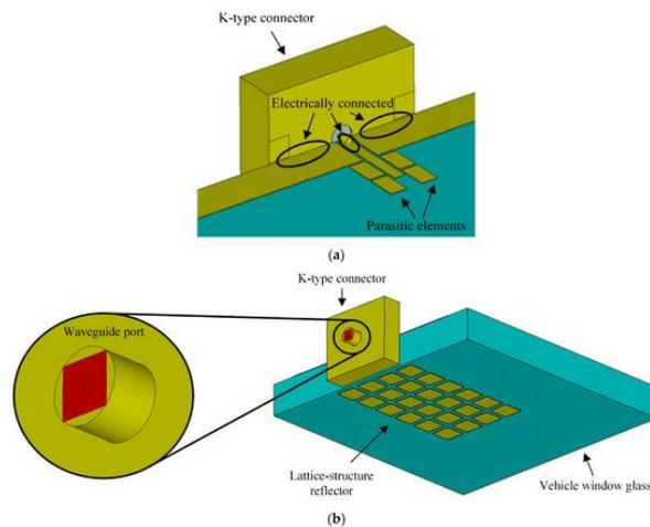
Figure 2. The real connector model in the CST EM modelling software with a waveguide port: (2) a waveguide port excitation portion, (3) a feeding connection component.
