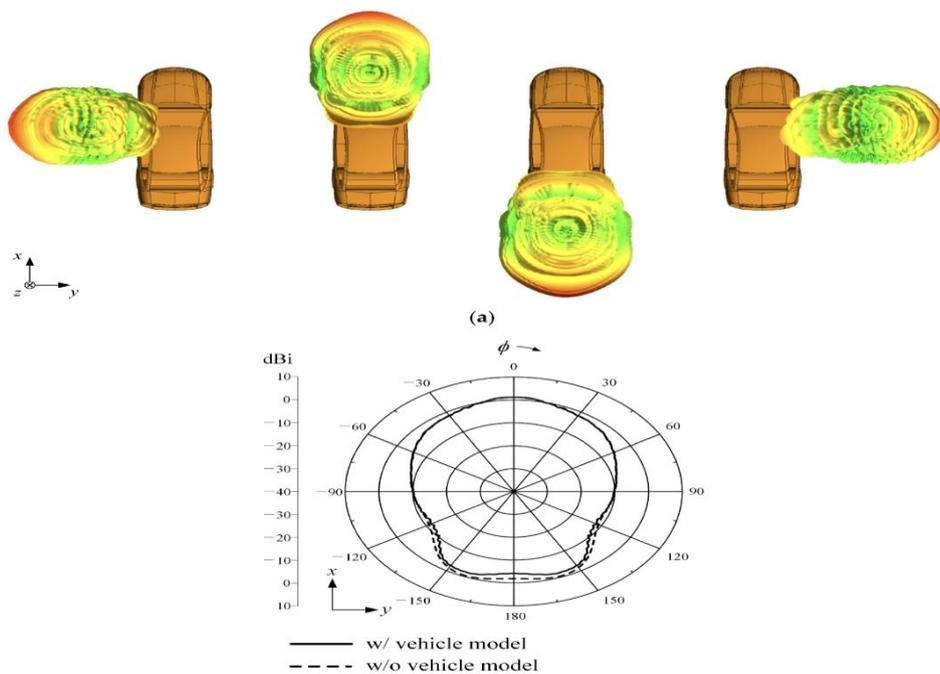
Figure. Simulated radiation patterns of the suggested antenna taking into account the impacts of the vehicle platform: (a) 2D radiation patterns with and without the vehicle mode, as well as 3D patterns based on the mount location.
