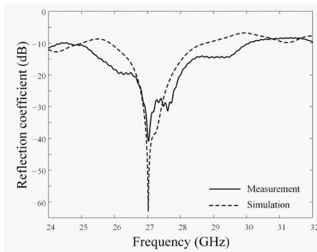
Figure 5 shows the proposed antenna's reflection coefficient.
