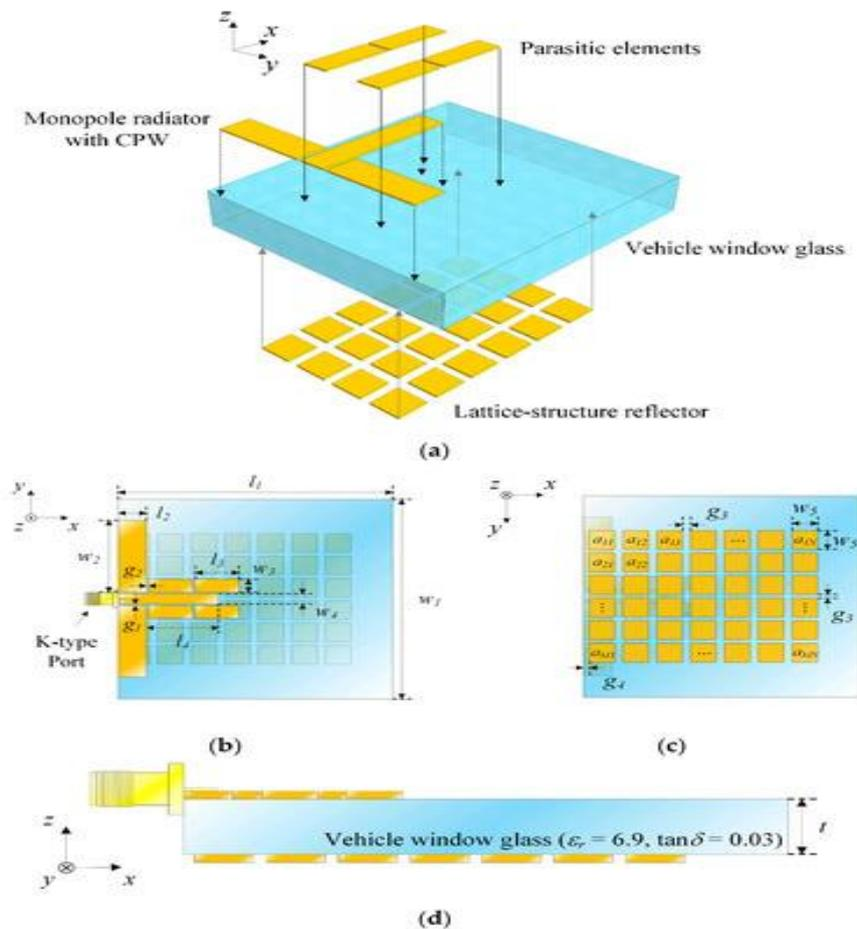
Figure 1 shows the proposed printed antenna's geometry in isometric, top, bottom, and side views.
