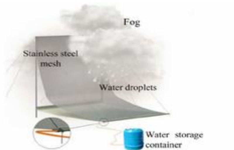
Fig 5 Fog Water Harvesting by Stainless Steel Mesh [22]
