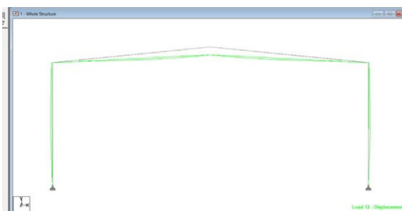
Fig 5 showing Displacements of the structure
