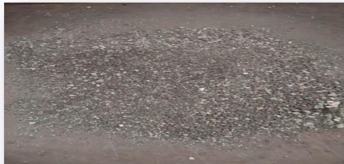
Figure 2. Black Cotton Soil Mixed with Silicon Manganese Slag
