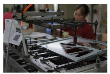
\*The side panel from the previous image is displayed here on a different manually operated machine. With this one, pilot holes are drilled in preparation for installation. If you look closely, you can observe the drillbits emerging from the machine's base.
