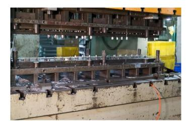
\*Every scrap of metal is being knocked out and is falling to the ground. The equipment seen in the previous image feeds metal via a tooling that is attached to a press.
