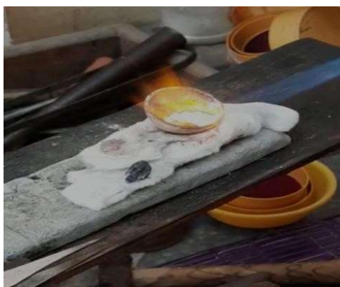
Fig-12: Burning silver precipitate using gas burner
