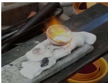
Fig-7: Burning the silver precipitate in a crucible using gas burner
