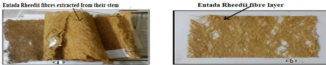
Fig. 5 (a) Entada Rheedii fibre layers extracted from their stem and (b) Single layer of Entada Rheedii fibre after washing with normal water
