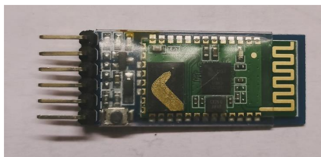
Fig.2. Pin Configuration of Bluetooth module front-view
