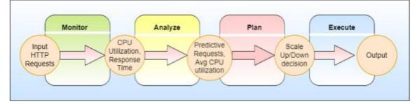
**Monitoring:** The monitoring system collects data via http requests from a cloud environment. Measuring web application performance is used to determine the best auto-scaling methods. CPU usage and request response time are taken into account.
