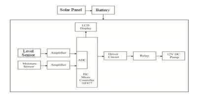
The above fig shows Microcontroller based irrigation system shows to be a real time feedback control system Which monitor sand controls all the actions of drip irrigation system competently. The present proposal is a Model to update the agriculture industries on a small scale with best expenditure. Using this system, onecan save manpower, water to advance production and ultimately profit.
