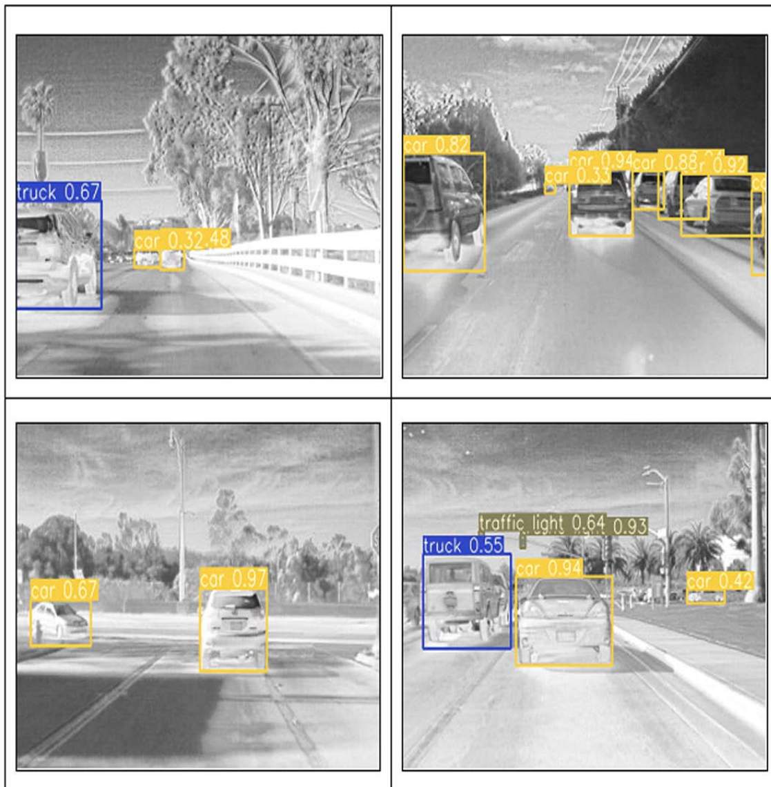
Figure 8. Vehicle Detection with bounding box using Yolov3 for certain image instances
