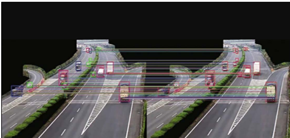
Figure 7. Features extracted by ORB algorithm for vehicle detection
