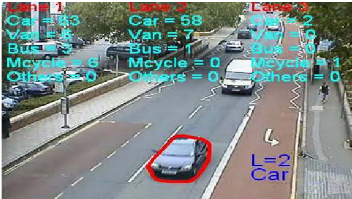
Figure 1. Vehicle detection and classification using deep learning: a deep learning perspective instance of an analytical image.
